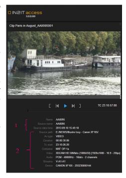
By clicking on the TimeCode (TC), the time reference changes display and becomes "abs TC", the display is then in minutes, seconds and frames from the beginning of the clip.
