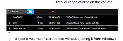
If an external volume is disconnected from the ingest station without being ejected through the application interface, and if the alert message is not validated, media are removed from the interface after 5 seconds.
